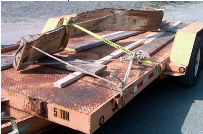
The first half of the coupling and recovered bolts from Shaft 5A have been removed and delivered to Altran's lab for testing.
